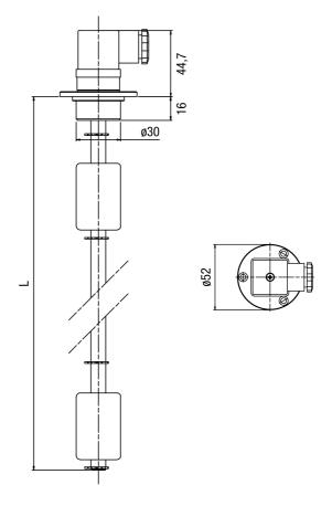
Level switch particularly suitable for hydraulics, lubrication plant, water treatment, industrial vehicles, fluid stocking, cleaning machines and equipment. The hermetically sealed reed switch housed inside the stem is actuated by a magnetic field created by a magnet equipped float. As the float rises and lowers with liquid level, the magnetic field passing the switch in the stem causes the switch to either open or close. Executions specifically approved R.I.N.A.
