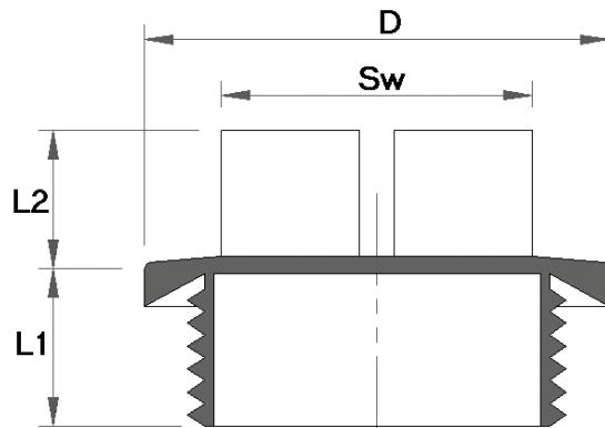
Threaded plug with hex head made to protect female hole,
