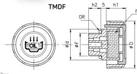
fb = Bronze filter f= Air filter OR = O-Ring NBR seal
